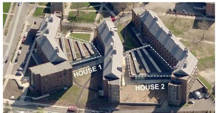
Figure 1 Research site. House 1 (left) is an intensive roof, and House 2 (right) is an extensive roof, both situated at Cornell University in Ithaca, New York. Campus image from Google Earth.
